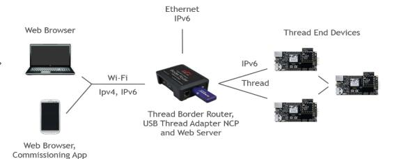
Figure 3: The Thread Border Router System Components with EFR32 Mighty Gecko Wireless SoC Starter Kit served as the basis of the analyzed test bed.
