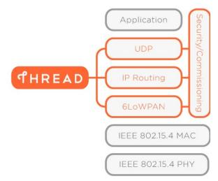
Figure 1: The Thread specification defines existing protocols and standards for various layers of the interconnect model, with implementation guidance primarily focused on the network and transport layer.
