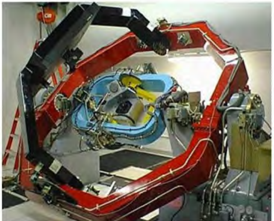
Figure 1: Five-Axis Flight Motion Table used in Scene Projection HITL
