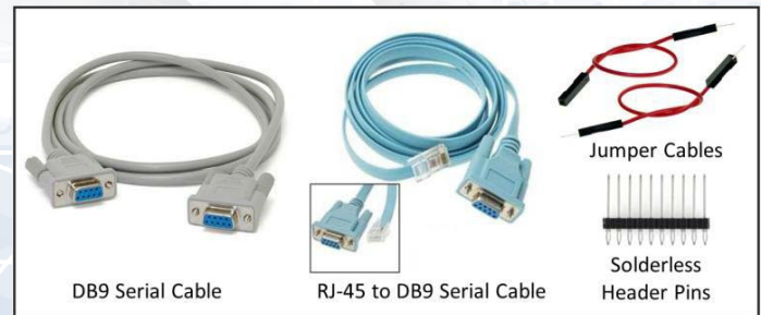
Figure 3: Cables and Wires - (Source: Author)
